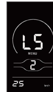
Fig. 7-2 Speed Limit Setting Interface
